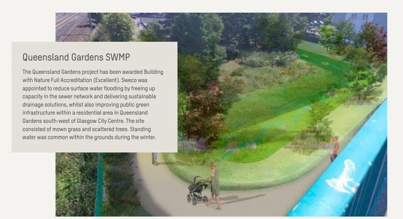
Within this project Sweco carried out flood risk assessment, drainage catchment analysis and design of new blue-green features comprising of an attenuation basin and swales around two blocks of flats.
